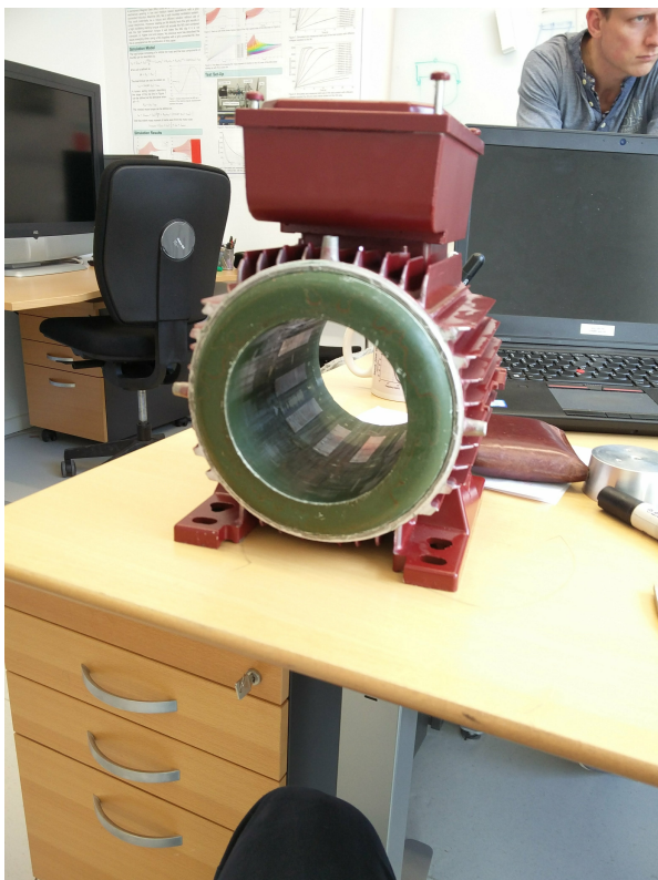
Figure 3.1: LeroySomer LSRPM90SL stator
